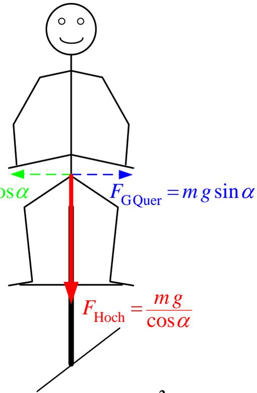
$$F_{G_{\text{quer}}} = F_{Z_{\text{quer}}} \Rightarrow \text{stabiler Fahrzustand} \Rightarrow \alpha = \arctan \frac{v^2}{g r}$$
